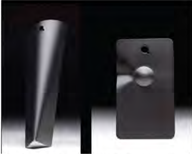
Figure 12. Unparalleled impact resistance assures increased durability while tight bend radii demonstrate good adhesion properties.
