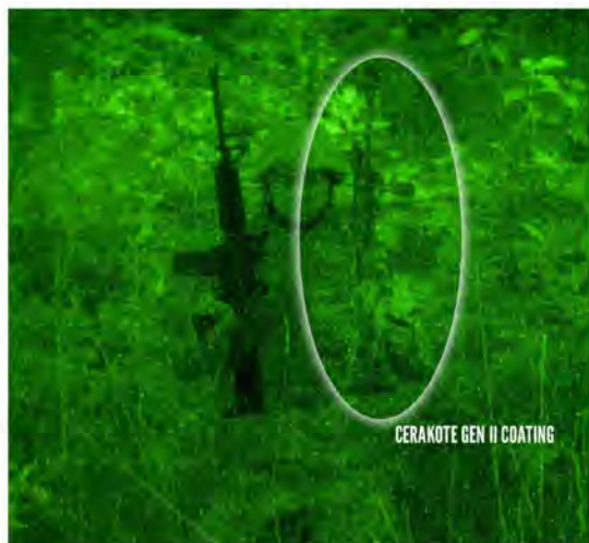
Figure 3. N-IR signature is managed by emulating the background reflectivity. The weapons on the right and top are coated with one of the products offered in the Cerakote™ Gen II line.
